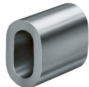
The Talurit® STS ferrule has a solid design which results in a powerful termination that remains safe and reliable even in the harshest conditions. The ferrule is made of special carbon steel that is specially treated to ease the cold-forming process. STS ferrules are typically used for applications that require resistance to mechanical wear, high temperatures, and corrosive environments.
